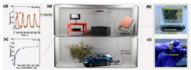
(a) Schematic illustration of the experimental steps to assess the concentration of NO x molecules from the vehicle emission using the mZFO sensor. (b) Prototype of mZFO based sensor to monitor the NO x concentration from vehicle exhaust. (c) mZFO nanoparticles coated on IDE with sensor casing. (d) The dynamic response after a few cycles of gas injection. (e) Laboratory collaboration data of mZFO sensor at different NO x concentrations.
